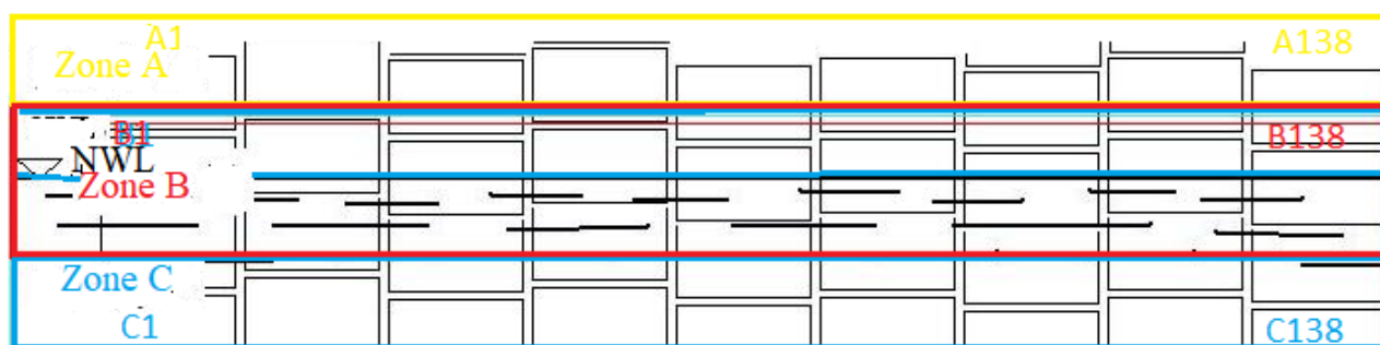
Fig. 2: Zoning of slabs (in vertical direction): zone A – above the changeable water level; zone B – at changeable water level (above or below NWL); zone C – zone under water (below NWL).
