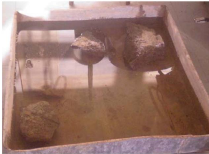
Fig. 4 Samples for estimation of concrete water absorption by weight W_m Source: compiled by authors
