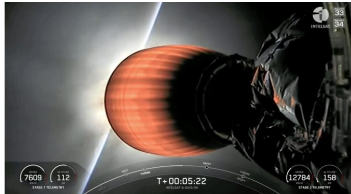
Fig. 3. Red-Hot SpaceX's Merlin Vacuum Engine (Zafar, 2022)
