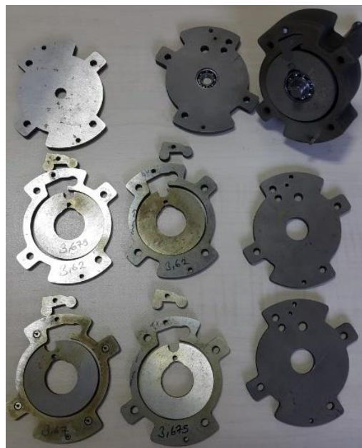
Fig. 3. Manufactured and Assembled Parts of the Compressor Source: Compiled by the author
