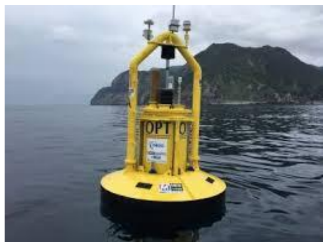
Fig. 8. Point absorber type WEC. Resource: [2]
