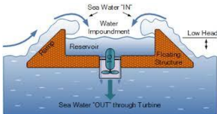
Fig. 5. Overtopping devices. Resource: [2]
